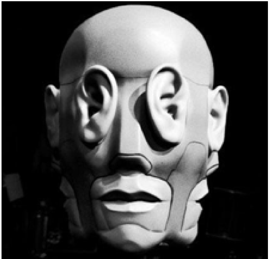
Image 2: Chris Milk's binaural audio recording instrument.
